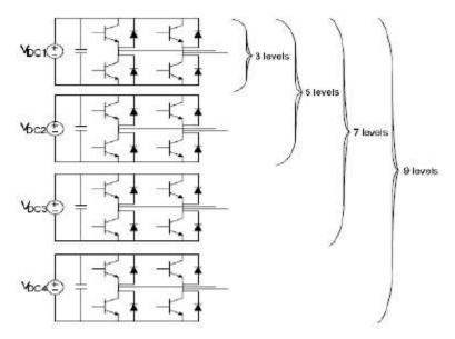
Figure 4(a) : Traditional cascaded H-bridge cell multilevel inverter (nine levels)
