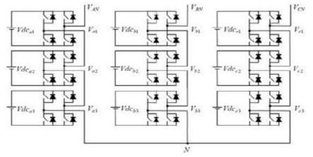
Figure 3: Cascade Multilevel converter
