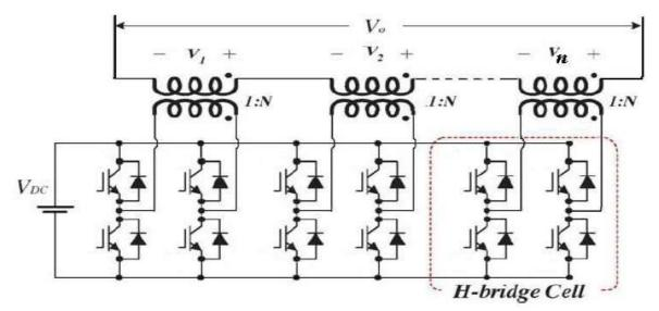
Figure 1: Circuit diagram of a single phase cascaded transformer H-bridge multilevel inverter
