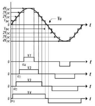
Figure 4(b): Operational waveforms
